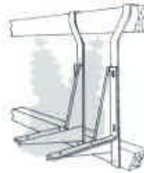
Figure 1—Vertical mounting with mounting brackets and hangers. Order as separate items mounting brackets style no. 463C035G02 and hangers style no. 261A233G01.
